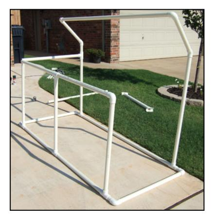
If you are happy with everything you can now remove the pipes from the fittings and begin gluing the pieces together. The PVC cement sets up really fast so you will have to be quick and accurate while gluing.
